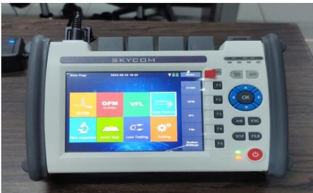
Gambar 2. OTDR (*Optical Time Domain Reflectometer*)
